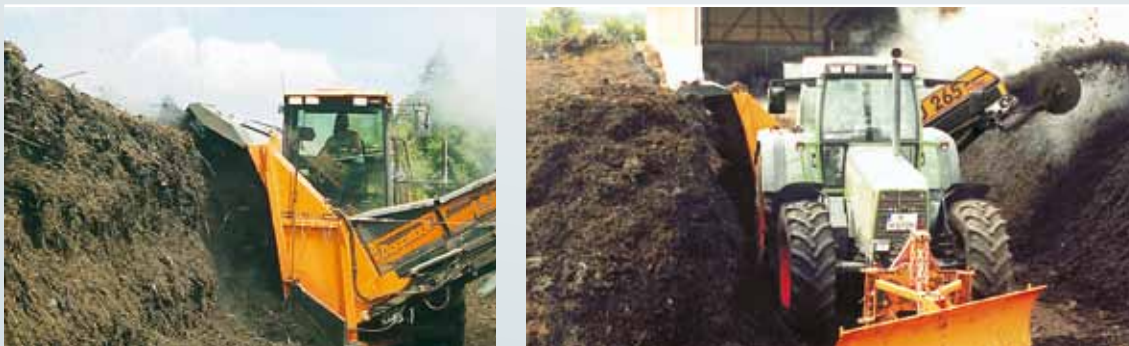
Turning and oxygen submission for windrows, contaminated soil and mechanic-biological installations
