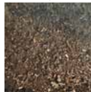
FINE FRACTION from the underflow of the second SELECTOR
